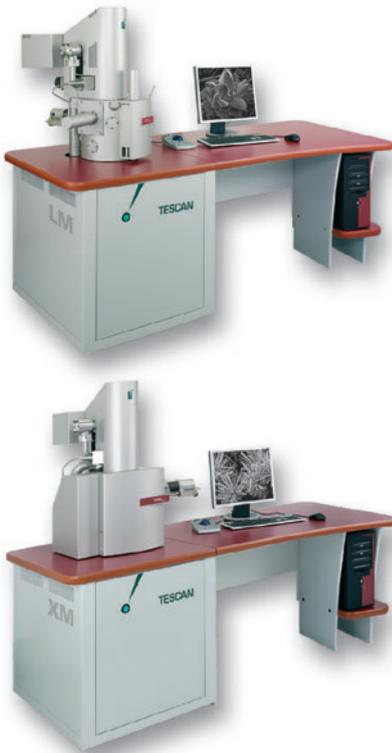
Following the most recent trends in nanotechnology research, Tescan has proudly introduced the new Mira series of high performance microscopes equipped with a Schottky field emission electron gun.
