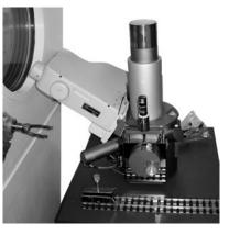
Remote controlled Tescan VEGA SEM placed in a "Hot Cell"
